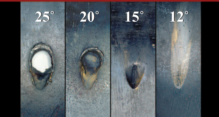
Test results using a 300 Win Mag Rifle
